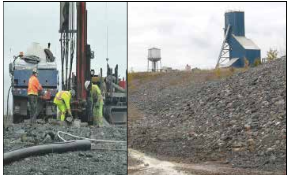
BacTech drills to test mineralization in concentrate stockpiled for over 50 years in Snow Lake, Manitoba prior to investigating feasibility of applying its proprietary bioleaching technology to clean up the toxic site and reclaim up to $150 million in gold contained in the ore.
